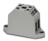
Device terminal block, Connection method: Screw connection, Number of positions: 2, Cross section: 0.5 mm² - 16 mm², AWG: 20 - 6, Width: 24.8 mm, Height: 40 mm, Color: gray, Mounting type: ct screw connection
